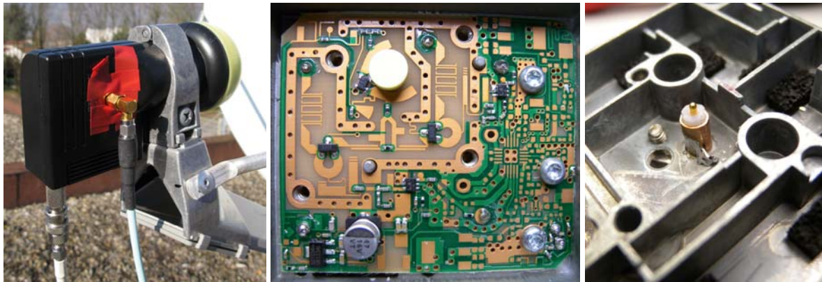
Figure 2: Technomate Low Noise Block downconverter. Left: LO injection on the body, middle: LO circuit with Dielectric Resonator Oscillator, Right: SMA connector that integrates a spring loaded contact for LO signal injection.
