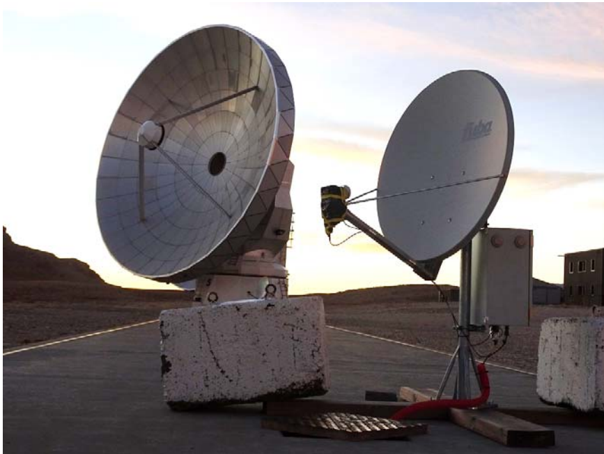
Figure 5: One Atmospheric Phase Monitor Antenna on E18 pad, next to a 15 meters NOEMA Array antenna.
