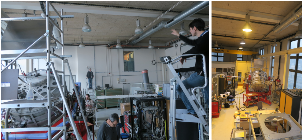
Figure 8 – (left) Photo of QUBIC in the foreground and the calibration source mounted on the wall at the far end of the room during the laser alignment procedure. (right) Photo of QUBIC looking along the line-of-sight from the calibration source. The reflection of the window is clearly visible in the flat mirror.
