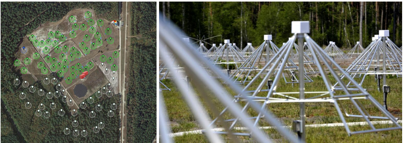
Figure 1 – Left picture: Satellite picture of NenuFAR. Green points are mini-arrays of 19 antennas. White points are future mini-arrays. Right picture: Picture of NenuFAR antennas (see [1]).
